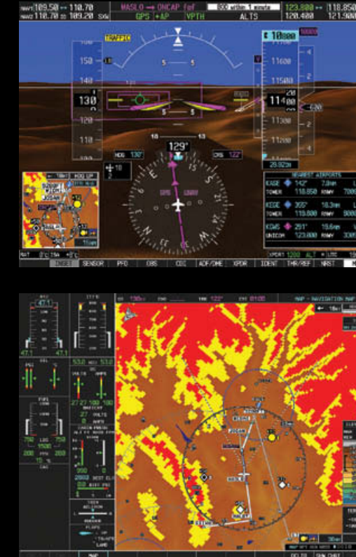
Optional Synthetic Vision Technology creates a 3D topographic landscape from the G1000's database. The resulting display depicts ground and water features, airports, obstacles and traffic all in relative proximity to your Mustang.
