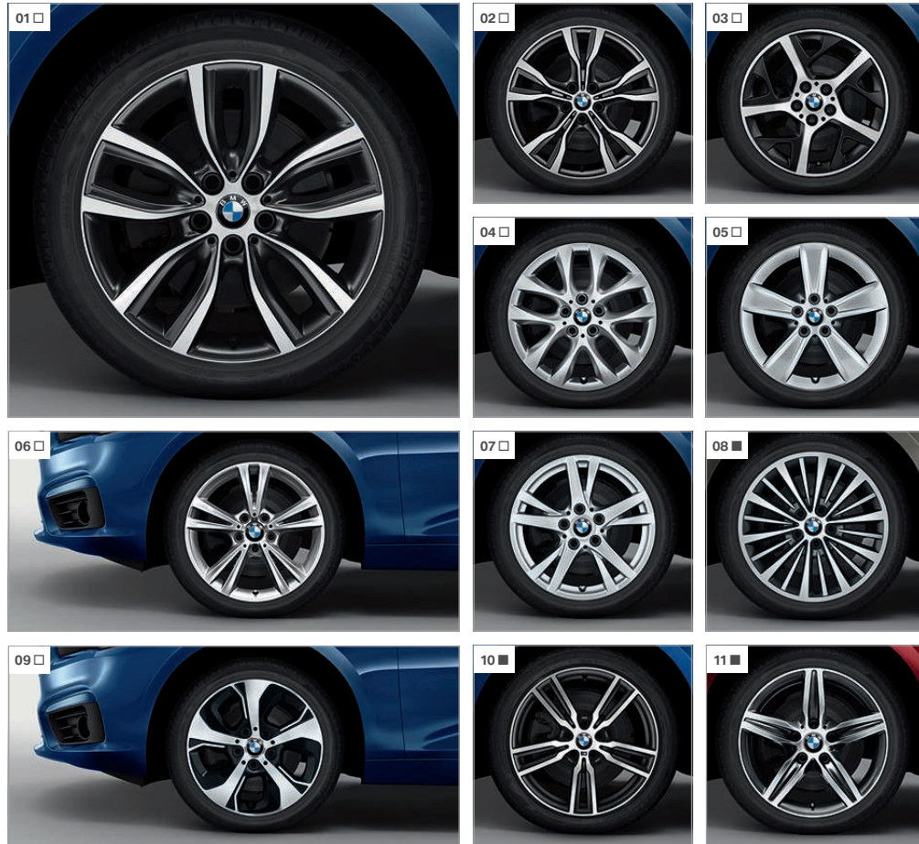
[ 01 ] 18" light alloy V-spoke style 485, 8J x 18 with 225/45 R18 tyres. [ 02 ] 18" light alloy Y-spoke style 484, 8J x 18 with 225/45 R18 tyres. [ 03 ] 17" light alloy Y-spoke style 480, 7.5J x 17 with 205/55 R17 tyres. [ 04 ] 17" light alloy V-spoke style 479, 7.5J x 17 with 205/55 R17 tyres. [ 05 ] 17" light alloy Star-spoke style 478, 7.5J x 17 with 205/55 R17 tyres. [ 06 ] 17" light alloy Double-spoke style 385 7.5J x 17 with 205/55 R17 tyres. [ 07 ] 16" light alloy Double-spoke style 473, 7J x 16 with 205/60 R16 tyres. [ 08 ] 17" light alloy Multi-spoke style 481, 7.5J x 17 with 205/55 R17 tyres (standard on Luxury models). [ 09 ] 16" light alloy Turbine style 472, 7J x 16 with 205/60 R16 tyres. [ 10 ] 18" light alloy M Double-spoke style 486 M, 8J x 18 with 225/45 R18 tyres (standard on M Sport models). [ 11 ] 17" light alloy Star-spoke style 379, 7.5J x 17 with 205/55 R17 tyres (standard on Sport models).
