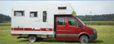
Our LB365 cabin on MB Sprinter is available for single and double-cab versions. In both cases, the vehicle can be equipped with our quick-mounting system, which enables quick and easy removal and mounting. Flat-beds or cargo compartments can be alternated with cabin for a truly dual purpose vehicle.
