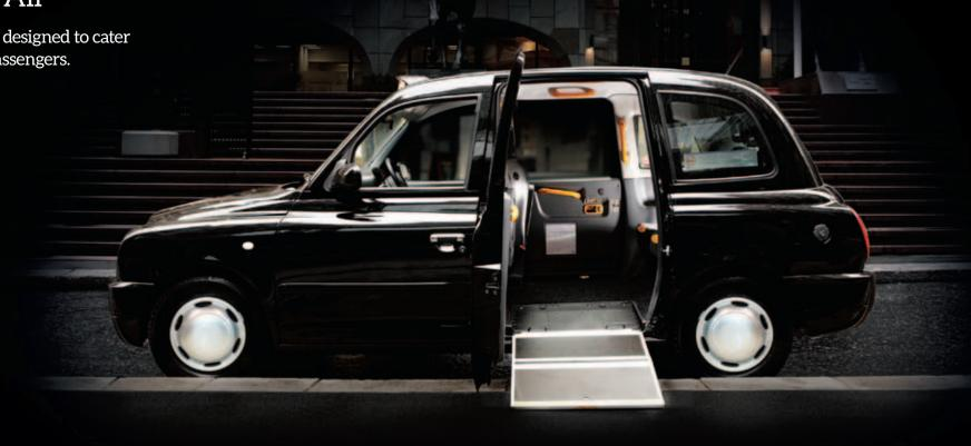
Integral ramps allow easy access, with a securing mechanism for wheelchair users providing stability during the journey.
