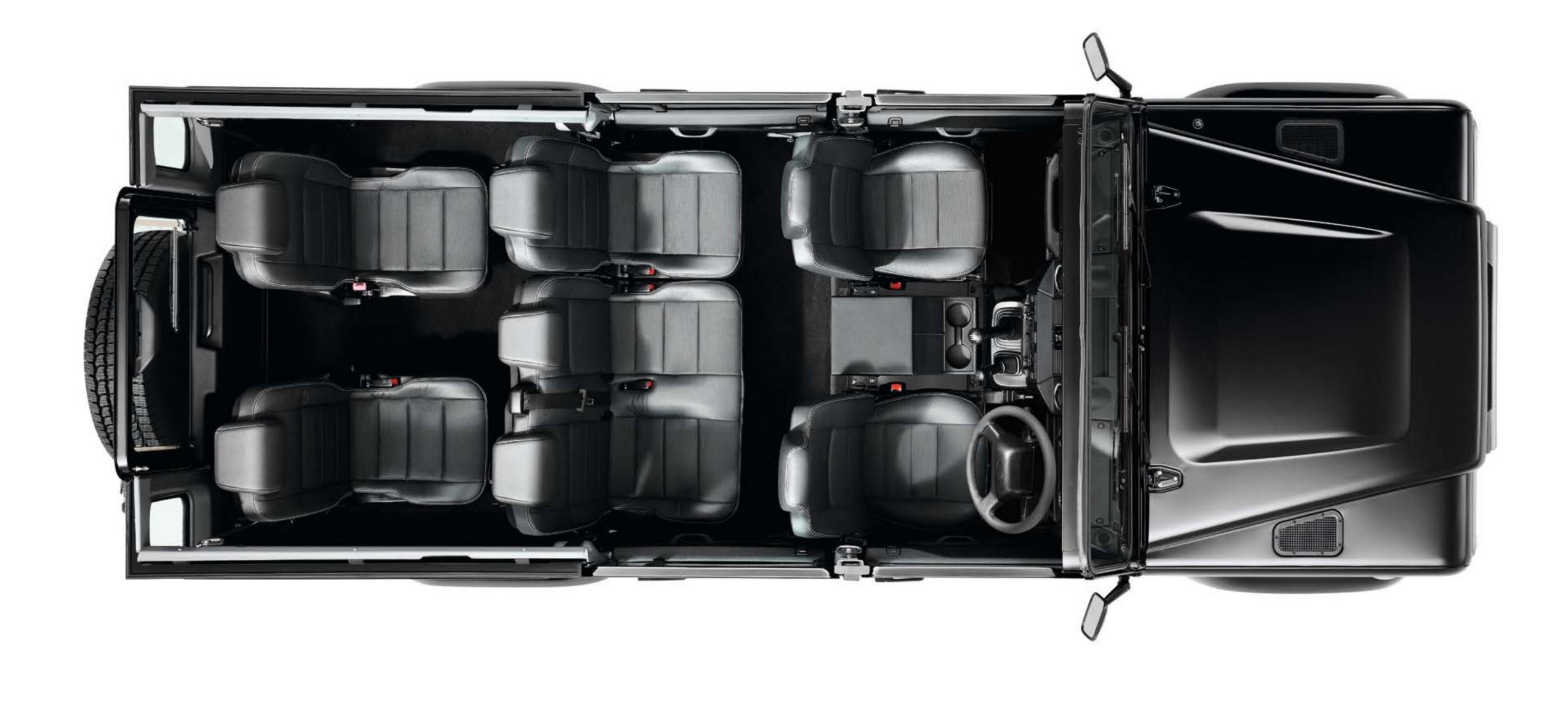
Form follows function in the Defender interior. Tough working vehicles demand robust materials such as the scuff-resistant facia and durable seat coverings. The facia is a one-piece moulding for improved refinement, its distinctive lines providing Land Rover's traditional commanding view of the ground ahead.
