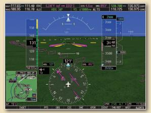
These magenta rectangular pathways provide a visual window to help pilots follow the intended flight route. Spaced no more than 1,000 meters apart, they have guidelines in each corner that point in the direction of the active flight plan leg.
