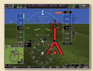
Using Synthetic Vision Technology (SVT), the Towers and Obstacles database makes awareness of non-terrain structural hazards crystal clear, even in low visibility.
