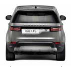
Front wheel track Air suspension 1,692mm Rear wheel track Air suspension 1,687mm
