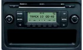
**Radio Blues:** CD player for audio CDs and MP3 audio files, AM/FM tuner with RDS system, convenient electronic encryption allowing operation only in a specific vehicle, amplifier power 4x 20 W (5J0 035 152A)
