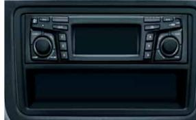
**Fitting kit** (AZO 700 001) and **cable adapter** (AZA 700 001A) are necessary for fitting a non-original radio into a car with a preparation for a Škoda radio.
