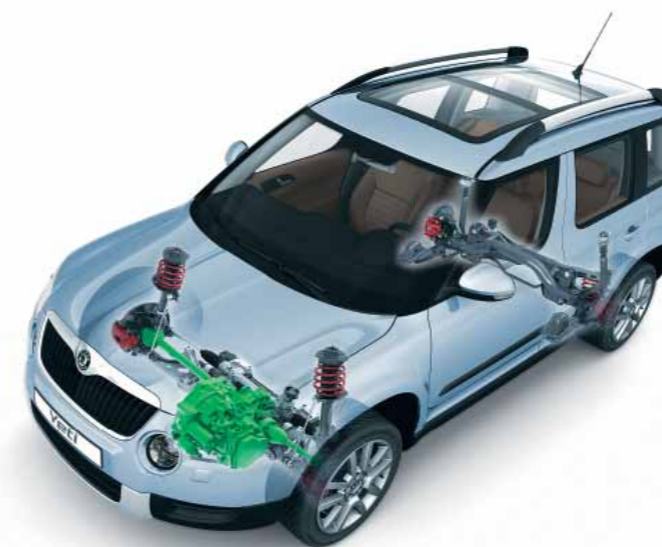
Škoda Yeti with a front-wheel drive (1.2 TSI/77kW; 1.4 TSI/90kW and 2.0 TDI CR DPF/81kW engines)
