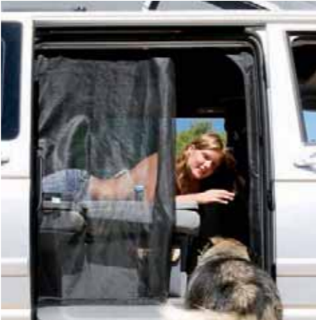
Fly net for sliding door. Net covers entire sliding door and can be unzipped to allow entry into the vehicle without removing it. Can be tied back when not in use.
