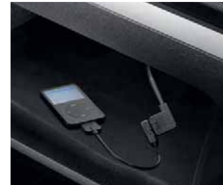
Media-in interface. Connect external audio sources such as MP3 Players, iPods, and USB-Sticks via the MEDIA-IN interface. Track listings can be viewed and selected via the vehicle's audio system. The unit also provides power to your media device and for iPods, charges your iPod whilst connected. Cables are purchased separately to suit your individual requirements.
