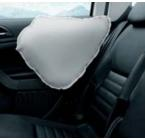
The rear side airbags, which are activated by a side impact, protect the pelvis and chest of passengers on the rear side seats.
