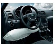
The driver knee airbag prevents contact with the lower part of the dashboard n the event of a collision.
