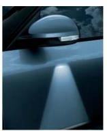
The **Boarding Spots**, designed to illuminate the entry area, are integrated in the external mirrors and enable you to avoid puddles and stones and so get in the car safely, even in complete darkness.
